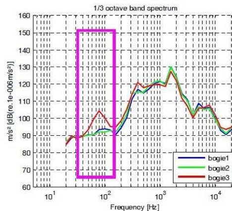
Time domain and frequency domain analysis is performed for each vehicle passage. The above example shows the time plot (top) of a vehicle passage, PSD plots and 1/3 octave band spectra plots for the three bogies of the vehicle. Both plots show a large wheel flat on bogie 3. The vibration levels for this bogie are clearly higher (more than 10 dB) than for the other bogie.
