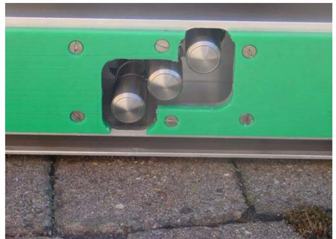
Figure 2: Three adjustable but equidistant contact making measurement probes with a large contact radius
