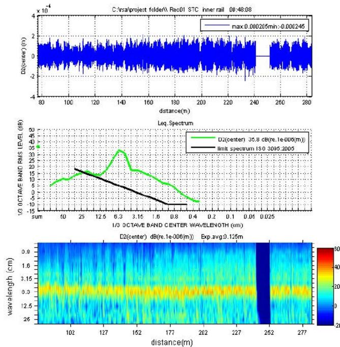
Figure 3: Typical measured roughness spectrum
