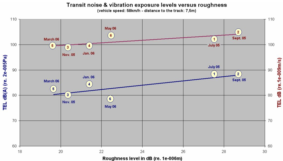
Figure 6: Transit noise and vibration exposure levels vs roughness at 7,5m from the track with a vehicle at 58 km/h.
