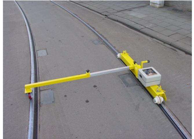
Figure 1: Rail Surface Analyser on embedded tracks and ballasted tracks
