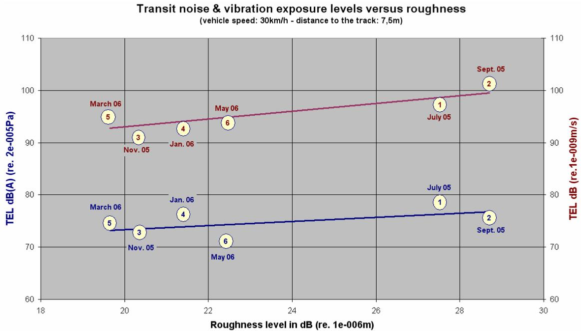
Figure 5: Transit noise and vibration exposure levels vs roughness at 7,5m from the track with a vehicle at 30 km/h.
